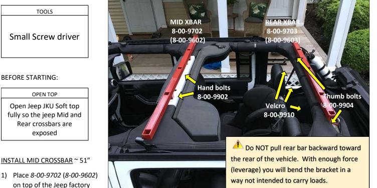
are facing down. Center crossbar. Use your Jeep Hardtop Hand Bolts from the underside up through the two holes that are approx. 15" apart. Hand tighten, but don't over tighten. (Hand Bolts come with your Jeep. Also sold separately if needed 8-00-9902)
